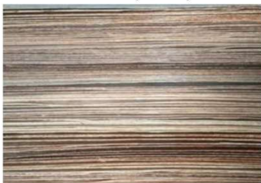
Figure 8: Peeled coconut veneer displays significant colour diversity from dark to light/pale brown
