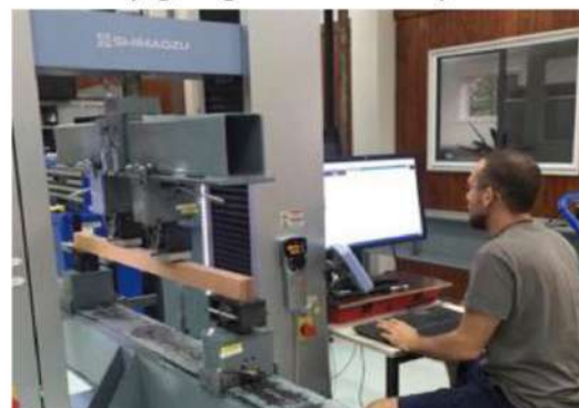
Figure 9: Coconut laminated veneer lumber (LVL) being tested for stiffness and strength.
