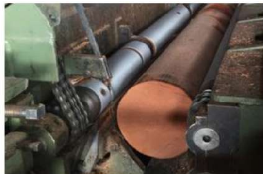
Figure 5: Harvested coconut stems being peeled using a spindle-less lathe
