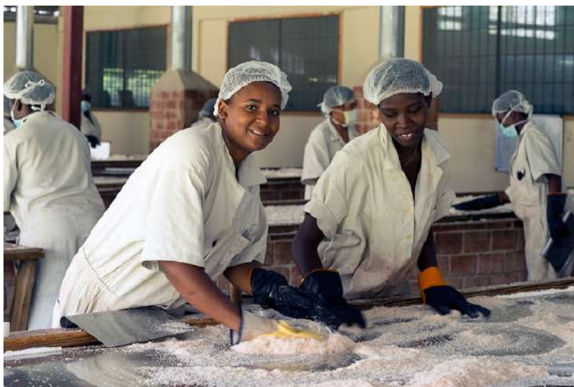
Drying grated coconut before being pressed using DME machine for VCO extraction
