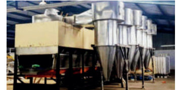
VIBRATORY FLUID BED DRYER
